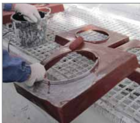
A CHIMNEY HOOD BEING MADE BY MANUAL LAMINATION
