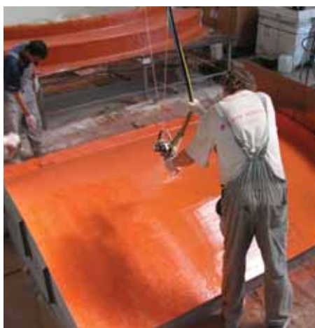
A CHIMNEY SEGMENT BEING MADE BY SPRAYING
