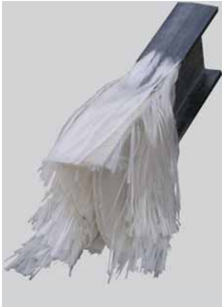
GLASS FIBERS REINFORCING A COMPOSITE PROFILE
